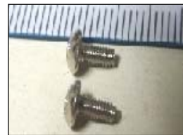
As for length of screw 6 mm
